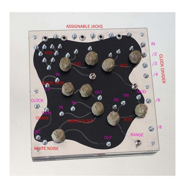
The three VCO's have all the same controls layout patch interface left to right Square , Triangle , Mod Input left knob - frequency right knob - Mod amount switch - frequency range select
